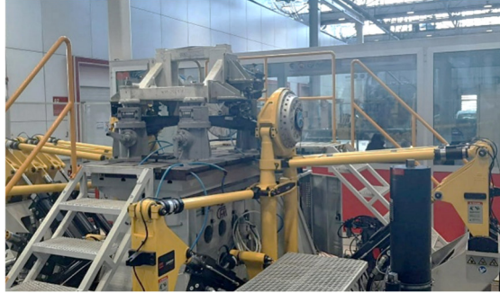
Figure 2: 6 Degree of Freedom Road Simulator used in the study.
