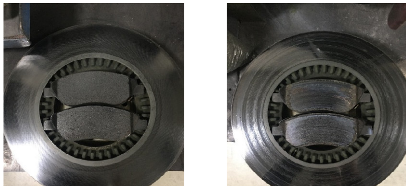
Figure 3. After the test the Cr3C2 coated brake disc and brake pads
